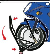
When the pin is located in the steering stem, with stand positioned as per diagram, start pushing the handle downard while sliding the wheels forward as indicated by the arrows.
