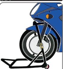
Once the rubber stoppers on the head lift stand have touched the floor, check to make sure the wheels are not moving and the bike is steady in place in the front and rear. When ready to remove the bike off the stands, always remove the front first, then the rear.
