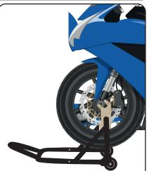
The rubber stoppers on the stand must be touching the floor once the propping motion is completed. Check all contact points and the pins for security before you start conducting any maintenance work.
