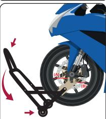
lifting pin (A) should be placed underneath the motorcycle front fork and lifting pin (B) resting behind the fork (As shown above).
