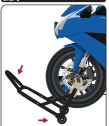
Once the front forks are correctly engaged by the paddock stand, push down on the handle while slowly sliding the stand wheels forward as indicated by the arrows above
