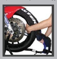
• When the wheel has fully rotated and the velcro end of the warmer has returned, pull the warmer firmly and secure the two ends of the warmer together. Make sure that heating areas of the warmer do not overlap each other. Make any adjustments to ensure the warmer is evenly located around the tyre – bunching, folding or overlapping of heating elements within the warmer will result in over-heating and damage to the warmer and tyre
