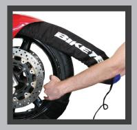
• When the wheel is fully rotated, undo the Velcro strap from the rim and remove the warmer fully. Immediately place the warmer on a dry surface, ensuring the warmer are fully extended, do not roll or fold the warmers together when they are still warm.
