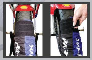
• Rotate the wheel away from you, feeding the warmer onto the tyre and ensure that it is evenly located and spaced. Take care when the warmer is passing through huggers or fenders - do not snag the warmer on any part of the bike (eg drive chain, sprockets). If necessary, loosen hugger or fenders to allow adequate access.
